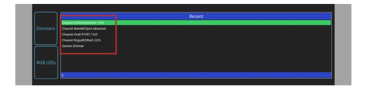
The 'Find Fixtures' option allows any fixture from the library of 23,000 fixtures to be quickly selected.
