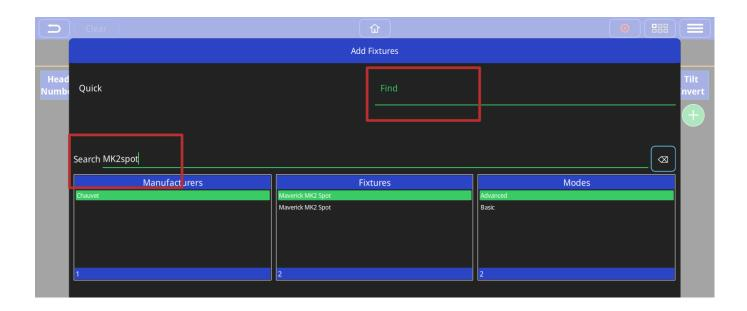
Once selected, enter the universe that the fixture(s) will be patched onto. Next enter the DMX start address of the first fixture.
