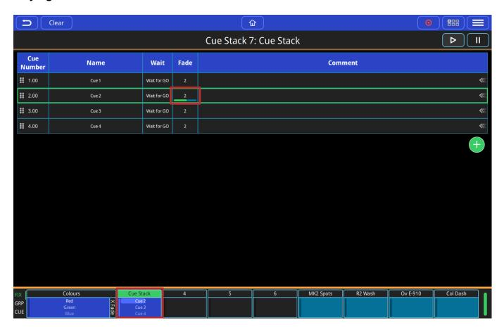
Selecting a playback by holding or double tapping on the cue stack preview above the fader will display the cue list on for that playback. Then. the GO Button on the console can be used to run the cues on the cue stack.
