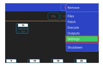
Also found within the QuickQ Settings window are a selection of global options that can be applied to the console, these can be found below the "Network", "DMX", "User Interface" and "Update" buttons. Changing the way the console playbacks, cue stacks and chases behave, QuickQ consoles can be run in 2 different modes, live mode and theatre mode.
