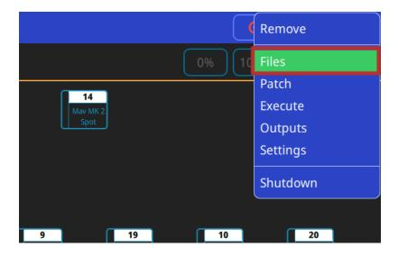
In the Files Menu, Press the 'New Show' soft button. This clears the current show file from memory – saved shows still remain stored on the console and can be loaded back into memory at any point, by selecting the 'Load Show' option in this window. Confirm by selecting yes.
