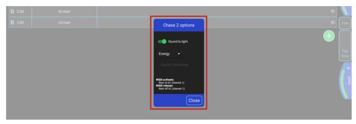
In this options window you can enable sound to light for this chase. You can also set the "Energy" option to look for specific audio frequencies. It this option is left as Energy, it will use the entire frequency spectrum.
