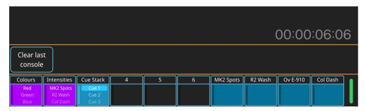
MIDI notes are pre-set on QuickQ with Playbacks 1-10 responding to MIDI notes 60 (C4) to 69 (A4). Simply send a note-on signal to launch and a note-off signal to release each Playback.
