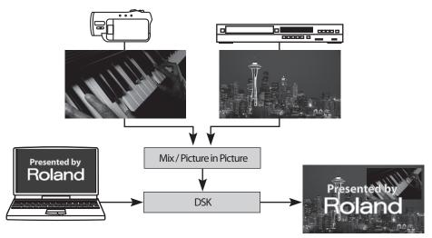
By default, the video on channel 4 is displayed in the foreground of DSK compositing. If you are using the unit with the default setting, input the logos and text to channel 4. To change the setting, refer to "Menu Operations and Menu List" (p. 45). Also, the extraction color for DSK compositing is set to black by default. You can use the menus to change this as well.
